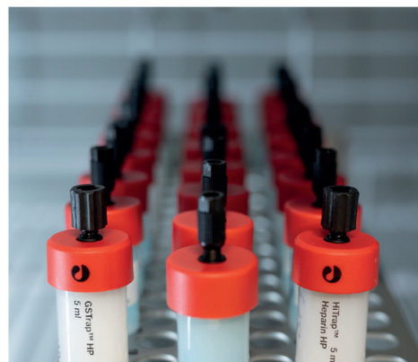
Figure 1. Left: Elution profile of a monoclonal antibody during the final gel filtration step. Plotted is the absorbance at 280 nm over the column volume (retention). The heavy and light chains of the antibody are visualised by Coomassie-stained SDS-PAGE next to the elution profile. Right: Various affinity and ion exchange chromatography columns used in the Core Facility.
